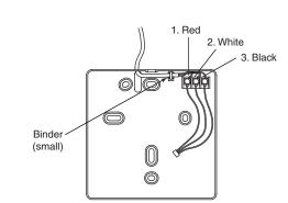
3. SETTING THE DIP SWITCHES When using a battery (memory backup)
