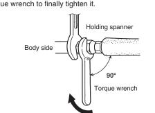
**↑** CAUTION Hold the torque wrench at its grip, keeping it in the right angle with the pipe, in order to tighten the flare nut correctly.
