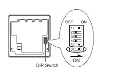
Change the DIP switch setting to use batteries. (The DIP switch is not set to use batteries at the factory.) Change DIP switch No. 6 from OFF to ON.
